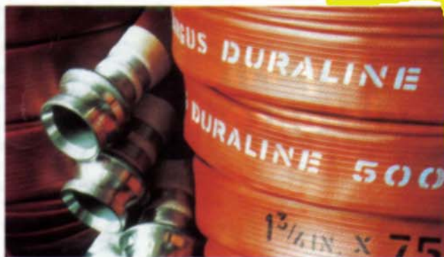
Duraline hose from Angus Fire is offered in lengths of up to 100 metres at diameters from 25-102mm. With a burst pressure of 50 bars and a safe working pressure of 21 bars, Duraline is able to meet the demands of higher nozzle pressures. Circle No. 128.
